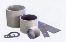
**HPF™/HPM™** filament-wound bearings combine the self-lubricating properties of PTFE with the high strength and stability of an oriented glass-fiber-filled epoxy resin backing. They provide high load capacities, excellent shock and edge loading resistance, low friction and wear, long service life and low water absorption for dimensional stability.
