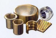
DB™ cylindrical, axial and self-aligning spherical bearings feature cast bronze alloy construction with graphite-free solid lubricant inserts. This structure provides an ultra-low coefficient of friction for greater wear resistance and longer service life than graphite-lubricated bearings.
