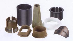
EP<sup>M</sup> series of solid polymer bearings provides low friction and excellent wear resistance. Made of a variety of engineering resins compounded with reinforcing fibers and solid lubricant, they exhibit excellent dimensional stability, high compressive strength and creep resistance, low thermal expansion and good thermal conductivity. These materials are available as standard parts or as customized solid polymer solutions.
