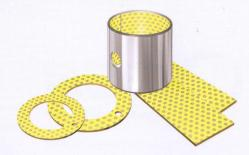
**DX**® prelubricated bearings feature a superior grease retention system for improved wear resistance and longer life in applications involving intermittent operation or boundary lubrication. Suitable for linear, rotating and oscillating movements, they provide optimum performance under relatively high loads and low speeds. The bearings also are available with plain sliding layers.
